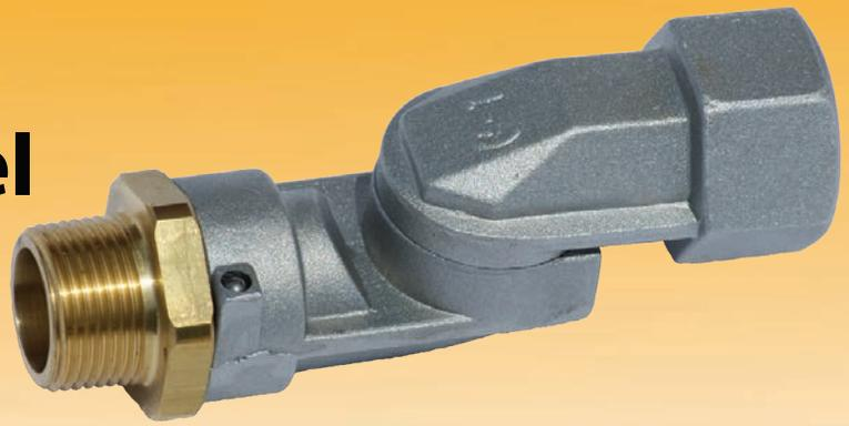
The construction of our new C1-2013 multi-plane swivel makes a dramatic departure from the standard practice in the industry. To provide the best surfaces from the O-ring seals to rotate on we have inserted a precisely machined sleeve into the aluminum castings. The sleeve is made from solid brass bar stock... the same material we use with the extremely successful single plane swivels.
